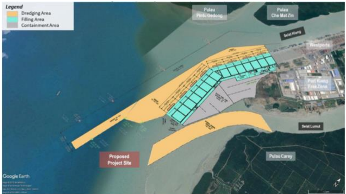
Figure 7 Proposed Dredging Area, Container Terminals and Containment Area
